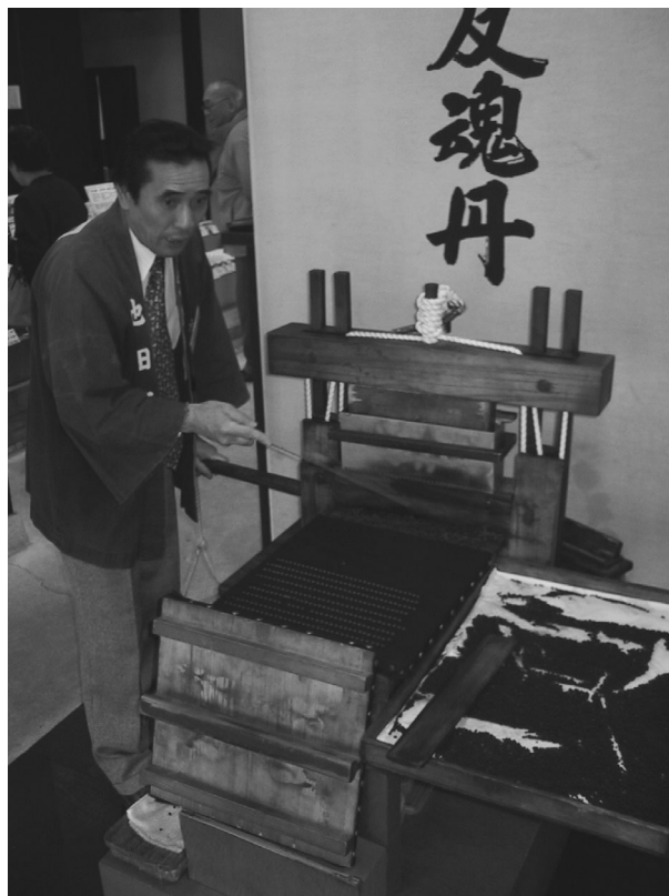
A traditional method of producing pills: pharmacist operating a mechanic, wooden machine
